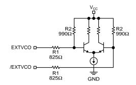
Figure 1. Simplified Input Structure
