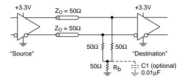
Figure 7. LVPECL Three-Resistor "Y-Termination" (Notes 1, 2, 3)
