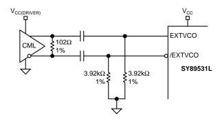
Figure 5f. CML AC-Coupled (Short Trace Lengths)
