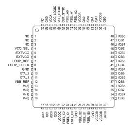
64-Pin EPAD-TQFP (H64-1)
