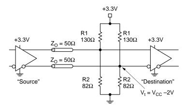
Figure 6. PECL Parallel Termination Thevenin Equivalent (Note 1)
