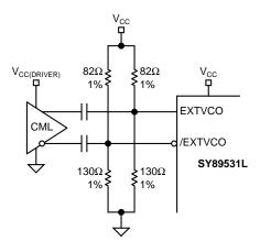
Figure 5g. CML AC-Coupled (Long Trace Lengths)
